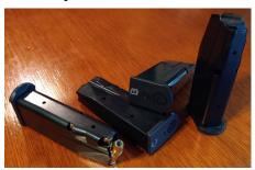
For those that run semi-automatic handguns (or other platforms that use a magazine), you should recognize and consider that magazines are the weak link in the chain. Typically, if a semi-auto stops working a majority of the time the culprit is in the magazine. This is why for Every Day Carry (EDC) we recommend always carry a spare magazine (it isn't all about just having more ammunition).
